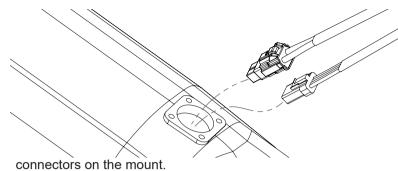
• Use 4 screws to fasten the charger cable onto the frame securely.
