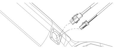
• Use 4 screws to fasten the charger cable onto the frame securely.
