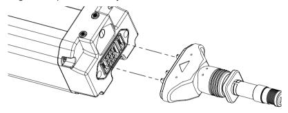
• Ensure battery and charger are same plane while charging via adaptor, to avoid adaptor to get loose.
