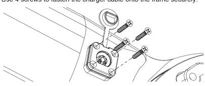
• Match the connectors on the charger cable with the corresponding connectors on the mount.
