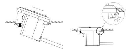
· Open the rubber cap and tighten the screws to the frame.
