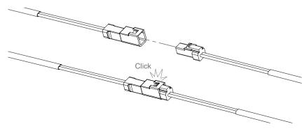
• Install the Y terminal (Red and Black wires) into the ACC slot of the motor.
