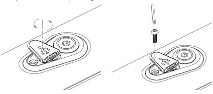
Match the connector on the button cable with the corresponding connector on the mount.
