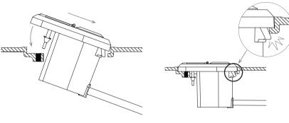
· Open the rubber cap and tighten the screws to the frame.
