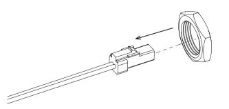
· Tighten the nut to the frame.
