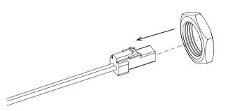
· Tighten the nut to the frame.
