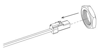
· Tighten the nut to the frame.
