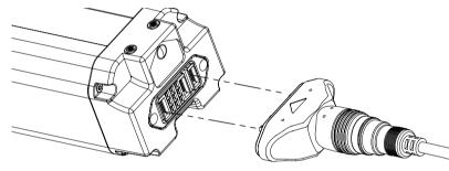
· Ensure the battery and charger are on the same plane while charging via the adapter to avoid the adapter from getting loose.
