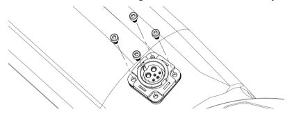
· Match the connectors on the charger cable with the corresponding connectors on the mount.
