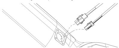
• Use 4 screws to fasten the charger cable onto the frame securely.
