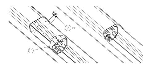
with screws. %The torque is 3N-M
